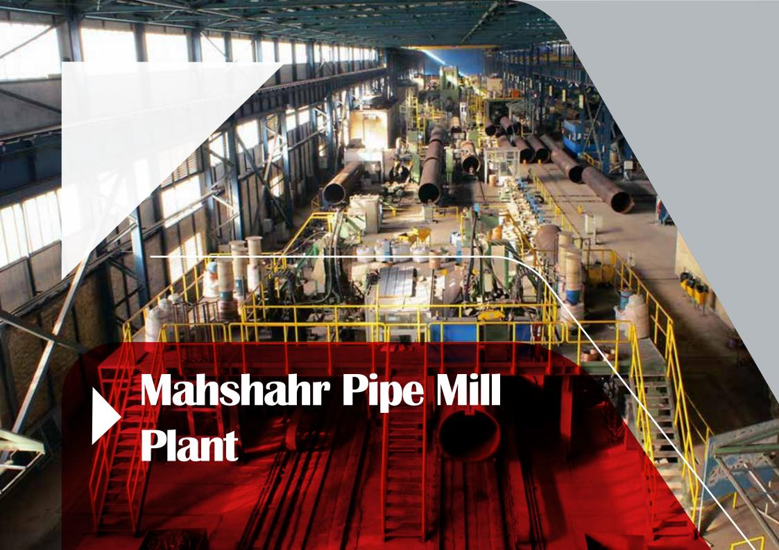
Largest Pipe Mill in the Middle East, Up to 56 inches Diameter and Up to 35 mm Thickness with 500,000 tons per year Capacity.
